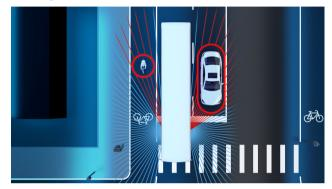
Sideguard Assist 2 is a safety assistance system that supports the driver in critical situations when turning right or turning left when visibility is possibly restricted. The system is designed to help detect moving obstacles within the system limits, and warns the driver so as to avoid critical situations or reduce the consequences of accidents when turning off or changing lanes.
