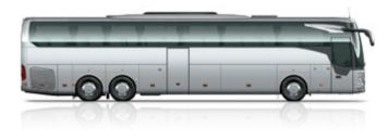
Length [mm]: 13.935 Turning circle [mm]: 23.327 Height [mm]: 3.680 Width [mm]: 2.550
