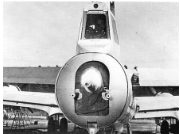
Figure 9-168h-5. Uncovered tall guns showing canvas turret boot and spent shell case chute beneath turret. The bomb release formation light is visible above the gunner's window.
