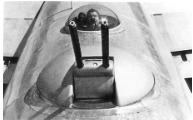
Figure 9-168h-3. CFC gunner in sighting position. Aft top turret reveals the camera port between the guns. A reinforcing fairing has been added around the turret.
