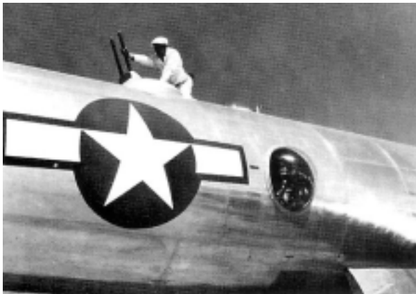
Figure 9-168h-2. Aft top turret and right sighting blister.
