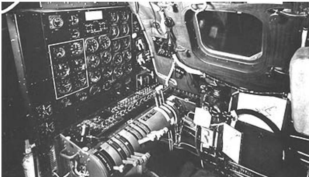
Figure 9-168e-2. The flight engineer's station was located directly behind the co-pilot. The seat faced aft. B-29 flight engineers during WWII were officers. Their skill at this station was soon appreciated by the pilots who learned to rely on them for getting the cantankerous R-3350 engines started and for nursing the crippled aircraft home.
