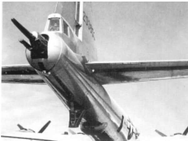
Figure 9-168h-4. Early tall gun installation with protective boots over the twin .50 caliber machine guns and the 20 mm cannon. This installation is on the first B-29A-5-BN.
