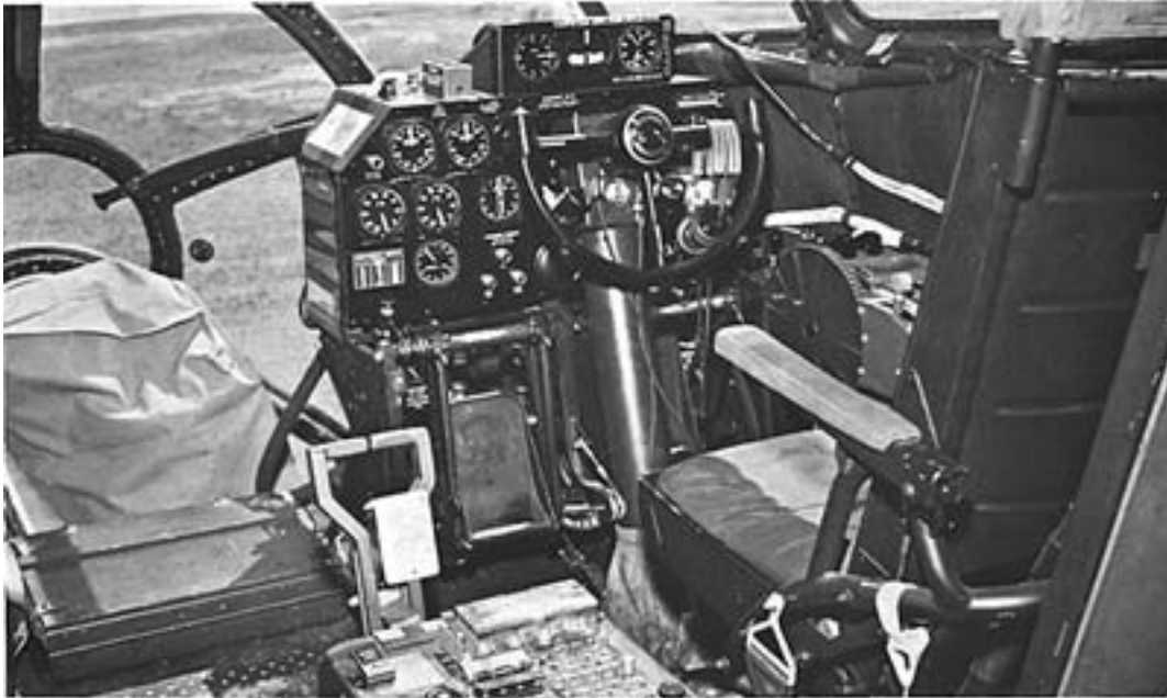
Figure 9-168e-1. Pilot's station showing aisle stand, controls, instruments, pilot's seat, and stowed bombardier's seat. Outside air temperature gauge is located on bombardier's greenhouse. Note nose glass deicing tube. 300 mph maximum airspeed placard is located above the flight instruments—airspeed, needle/ball, and rate of climb.
