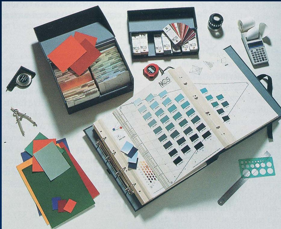
There are 40 constant hue triangles spaced at 10 'percent' change of the four fundamental hues.
