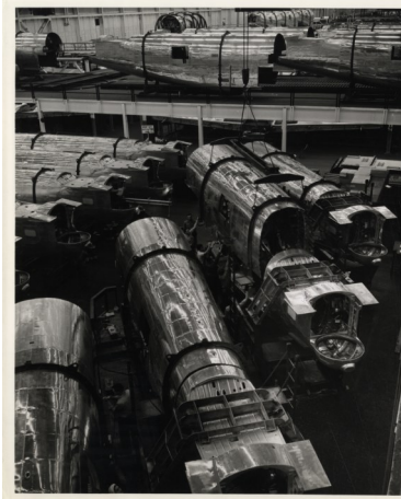
View of fuselages for the B-24 Liberator bomber at the Ford Motor Company Willow Run Plant . Courtesy of the Detroit Public Library
