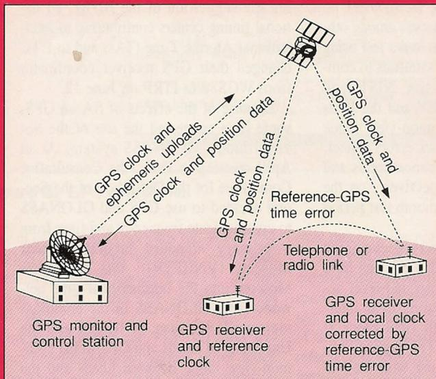
Figure 5: GPS common-mode common-view time transfer
