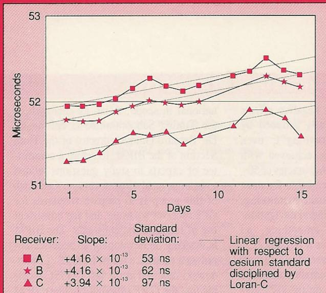
Figure 4: GPS 1PPS phase control
