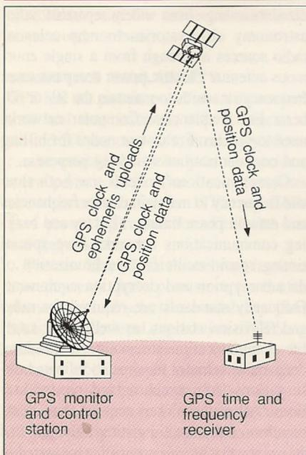
**Figure 1.** GPS time and frequency transfer
