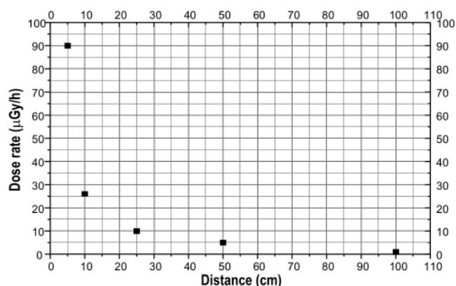
Figure 1. Depleted uranium ammunition caliber 30 mm external exposure of whole penetrator
