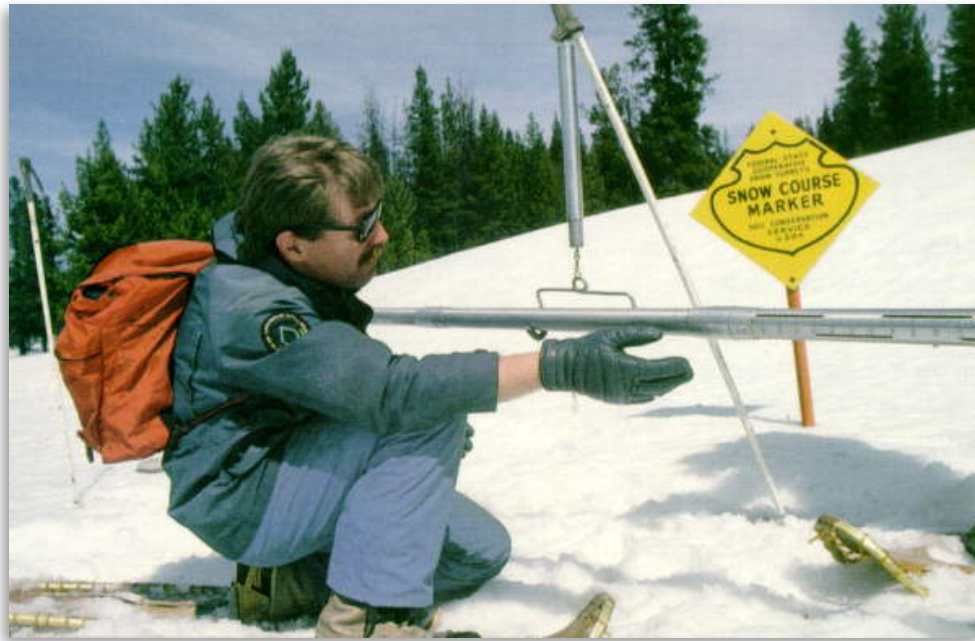
Figure 6. After clearing out any soil from the tube, the surveyor determines the amount of water in the snowpack by weighing the tube with its snow core and subtracting the weight of the empty tube. Source: NRCS ( www.wcc.nrcs.usda.gov/factpub/sect_4a.html )
