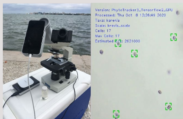
Left Photo: The HABscope system in the field. Right Picture: shows the AI program identifying Karenia brevis with the green squares. Image Credit: Mote Marine Laboratory and Robert Currier.
