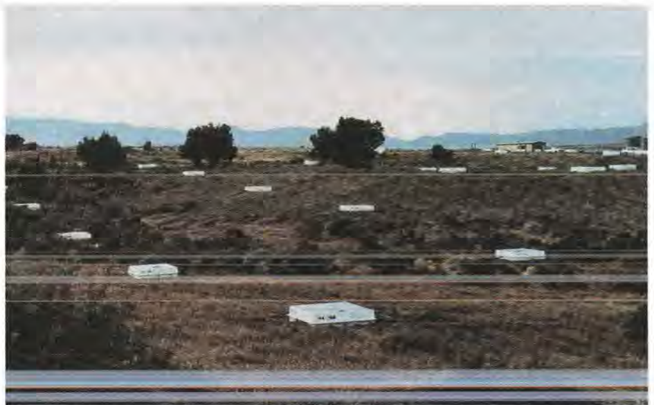
Chicago Air Shower Array. Shown here are some of the CASA scintillation-detector stations installed at Dugway, Utah. The stations are positioned on a square grid and measure discrete sources of ultrahigh energy cosmic rays. The completed array will consist of 1000 such detectors.
