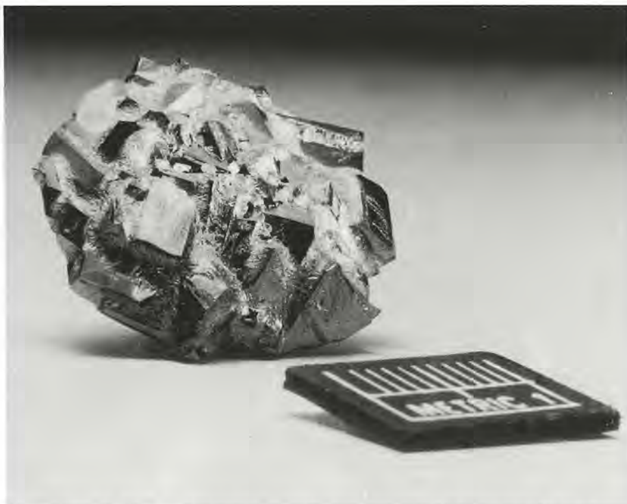
Material growth. Photograph shows pure lanthanum copper oxide grown on a platinum seed—a project of MIT's Materials Research Laboratory. The crystal has a layered structure that forms the basis for high-temperature superconducting materials such as lanthanum barium copper oxide.
