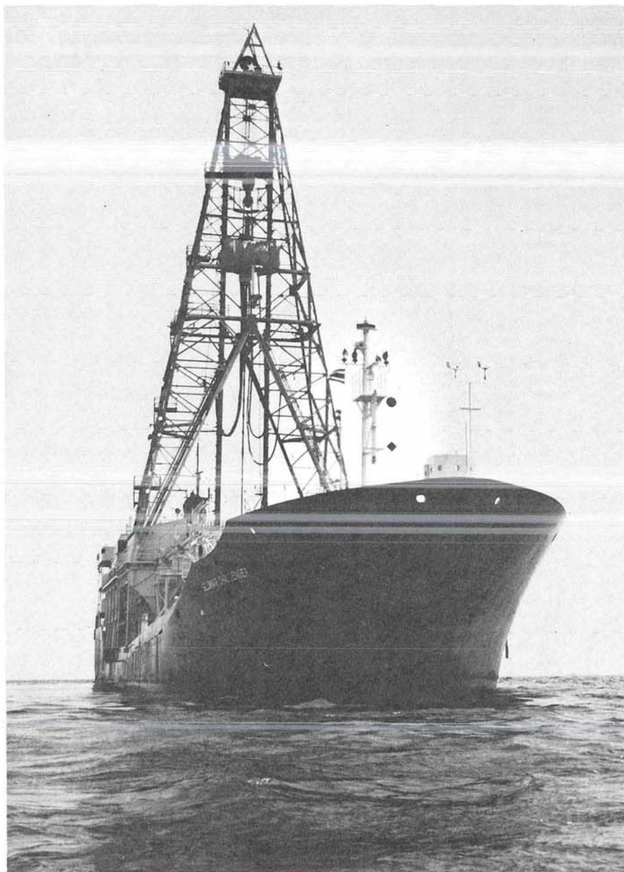
Glomar Challenger. Researchers are using this vessel for subbottom coring in the Deep Sea Drilling Project, which has drilled in all the world's major ocean basins. There were seven research trips, or legs, in fiscal year 1982.
