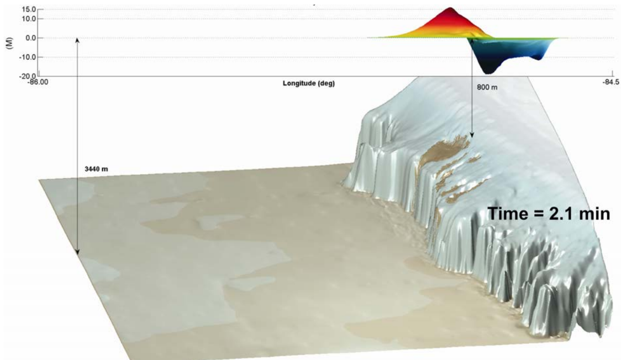
Figure 39. TSUNAMI3D's numerical result side-view for the West Florida submarine landslide. Maximum wave height recorded at 2.1 minutes after the landslide initiation.
