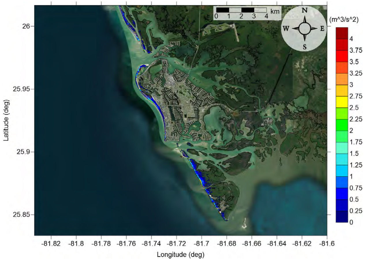
Figure 48: Maximum momentum flux ( \text{m}^3/\text{s}^2 ) caused by the Probabilistic Submarine Landslide B2 in Marco Island, FL. Arrows represent direction of maximum momentum flux. Contour drawn is the zero-meter contour for land elevation.
