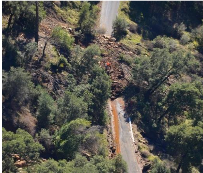
FIGURE 20: POST-WILDFIRE DEBRIS FLOW DEPOSITS ON A ROADWAY, CALIFORNIA.
