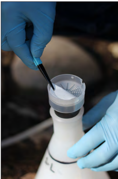
Figure 1.7. Method for folding filter paper in one-half four times using sterile forceps and clean gloves.
