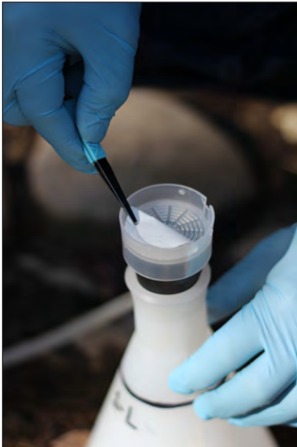
Figure 2.7. Method for folding filter paper in one-half four times using sterile forceps and clean gloves.
