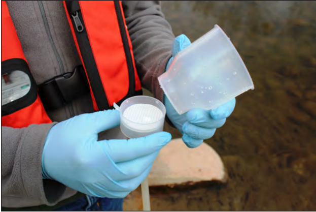
Figure 1.6. Disconnected top and bottom units of filter funnel and exposed filter membrane.
