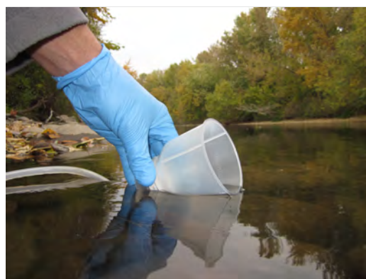
Figure 3.4. Filter funnel being submerged directly into stream with pump engaged to begin filtration.
