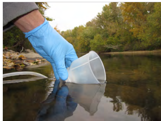
Figure 2.4. Filter funnel being submerged directly into stream with pump engaged to begin filtration.
