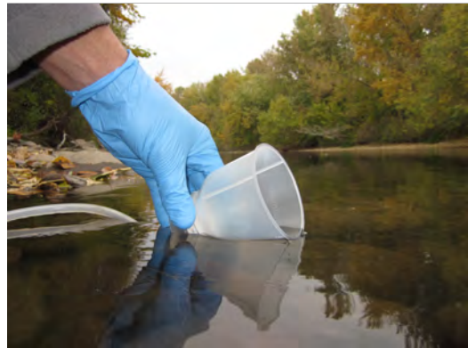
Figure 1.4. Filter funnel being submerged directly into stream with pump engaged to begin filtration.
