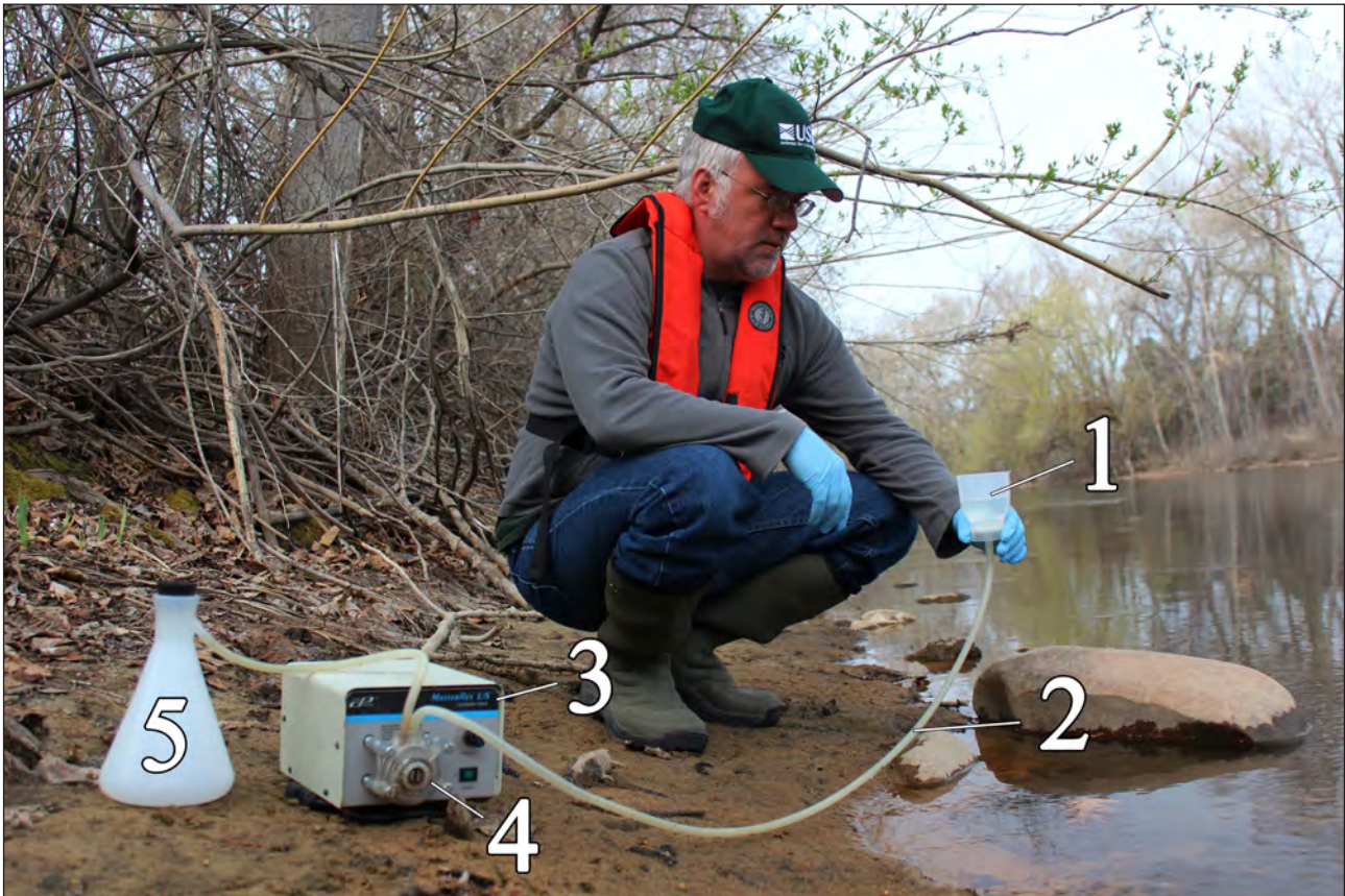
Figure 3.1. Necessary equipment: 1, filter funnel; 2, Masterflex® L/S 15 silicone tubing; 3, 120-V Masterflex® L/S economy variable speed drive motor; 4, Masterflex® standard pump head for L/S 15 tubing; 5, Nalgene™ vacuum flask. Note: See appendix A for manufacturer's information.
