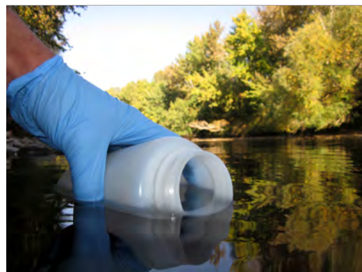
Figure 2.5. Sterile Nalgene™ collection bottle being submerged in stream to collect desired volume of water. Sample must then be poured into filter funnel (250 milliliters at a time) with pump engaged to begin filtration.
