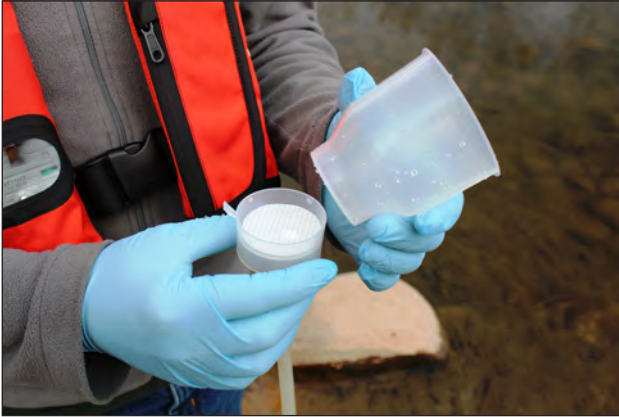
Figure 2.6. Disconnected top and bottom units of filter funnel and exposed filter membrane.
