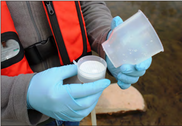
Figure 3.6. Disconnected top and bottom units of filter funnel and exposed filter membrane.
