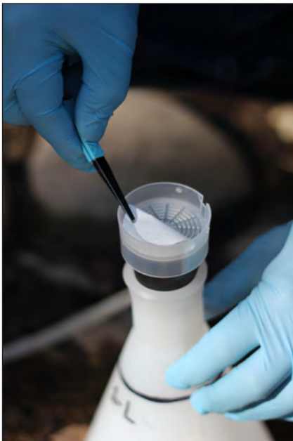
Figure 3.7. Method for folding filter paper in one-half four times using sterile forceps and clean gloves.
