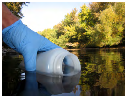
Figure 3.5. Sterile Nalgene™ collection bottle being submerged in stream to collect desired volume of water. Sample must then be poured into filter funnel (250 milliliters at a time) with pump engaged to begin filtration.
