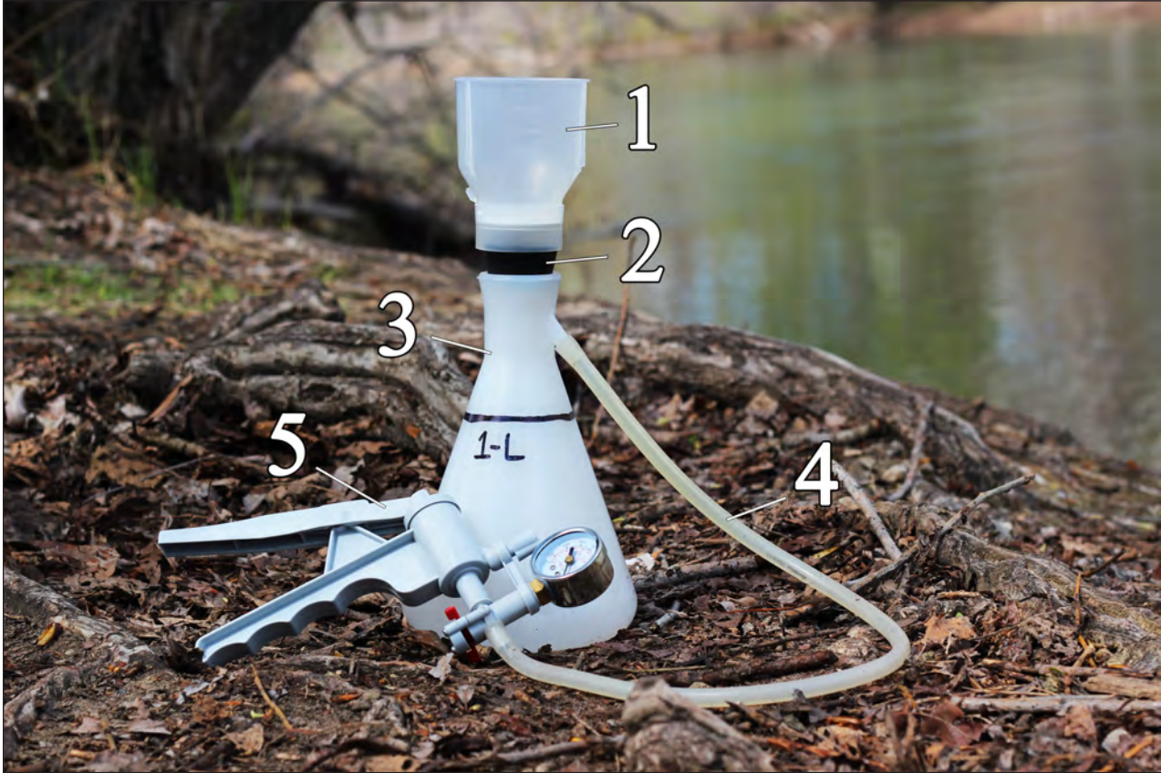
Figure 1.1. Necessary equipment: 1, filter funnel; 2, #8 Fisherbrand™ rubber stopper; 3, Nalgene™ vacuum flask; 4, Masterflex® L/S 15 silicone tubing; 5, Nalgene™ hand-operated vacuum pump. Note: See appendix A for manufacturer’s information.
