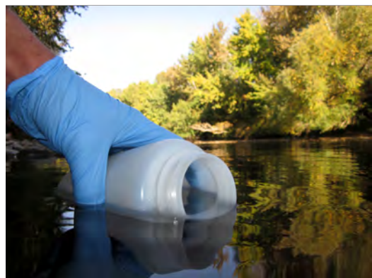
Figure 1.5. Sterile Nalgene™ collection bottle being submerged in stream to collect desired volume of water. Sample must then be poured into filter funnel (250 milliliters at a time) with pump engaged to begin filtration.
