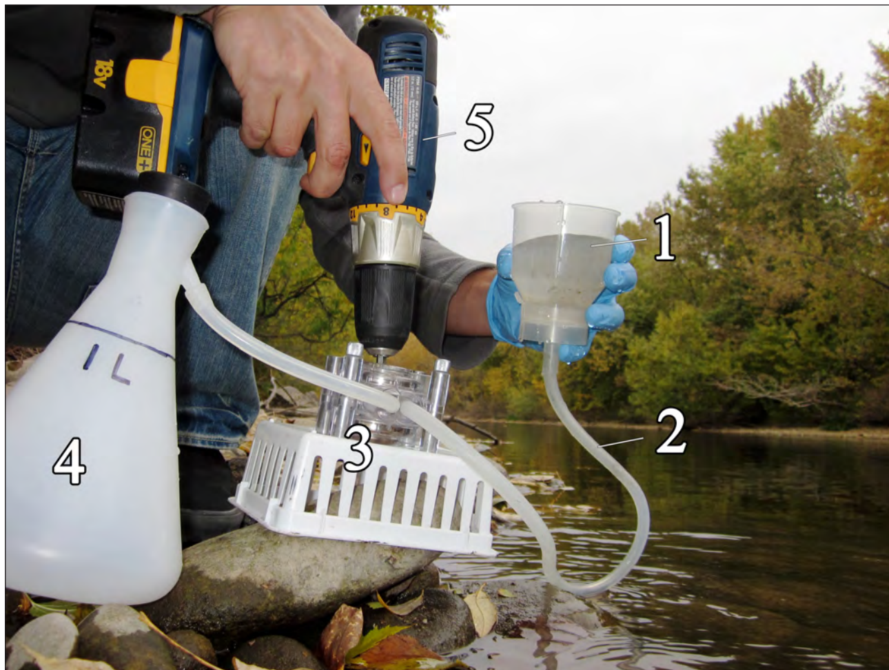
Figure 2.1. Necessary equipment: 1 , filter funnel; 2 , Masterflex® L/S 15 silicone tubing; 3 , Masterflex® standard pump head for L/S 15 tubing (shown mounted to piece of plastic); 4 , Nalgene™ vacuum flask; 5 , battery-operated driver/drill. Note: See appendix A for manufacturer's information.
