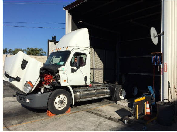
TTSI Running the Beta Engine on the Dyno
