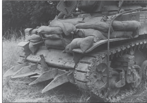
Close up view of Sgt. Culin's improvised hedgerow cutter attached to the front of an M5 Stuart light tank.
