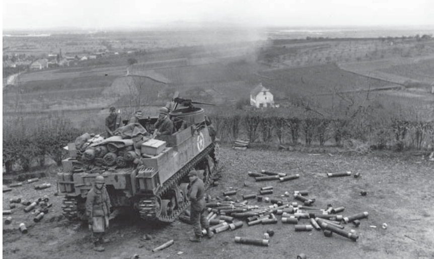
A 105-mm M7 Howitzer motor carriage shells German positions in the Rhine Valley.
