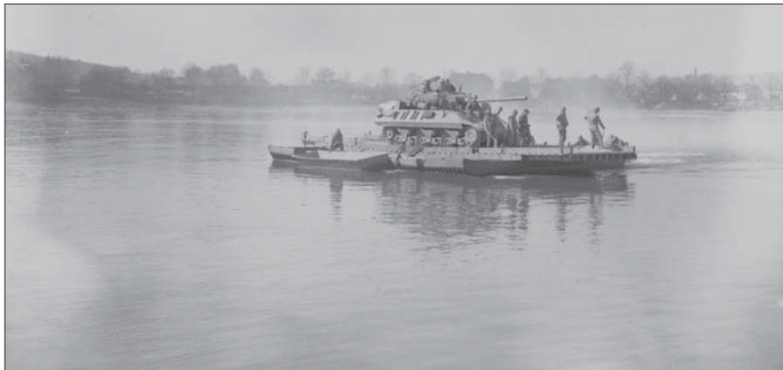
An M36 Tank Destroyer crosses the Rhine on an assault boat raft.
