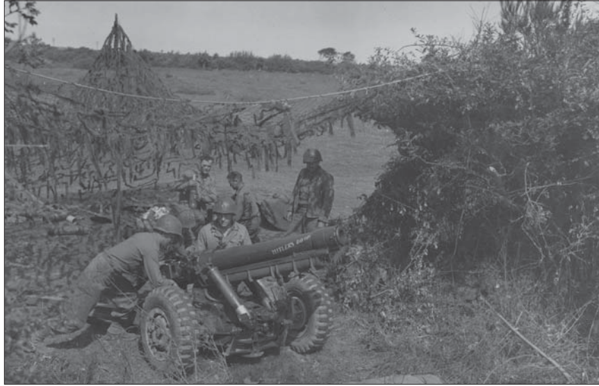
"Hitler's Doom," a 105-mm M3 howitzer, being sighted in at the siege of Brest.
