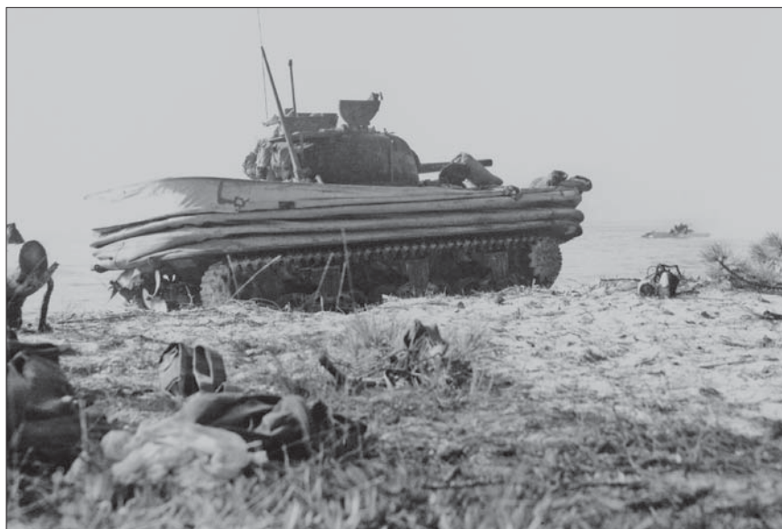
A Duplex Drive tank with its separate amphibious propeller drive and canvas waterproof screen.
