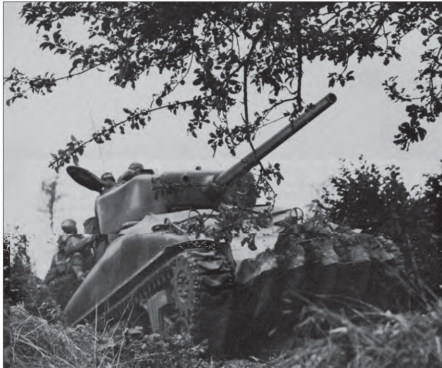
An M4A1 Sherman medium tank busts through the bocage with the help of a hedgerow cutter.
