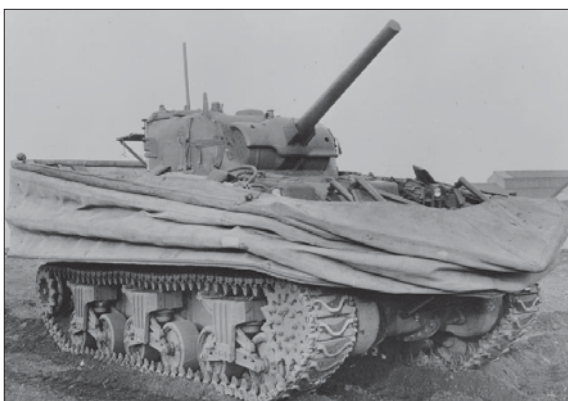
A dual drive tank with its canvas flotation screen lowered.
