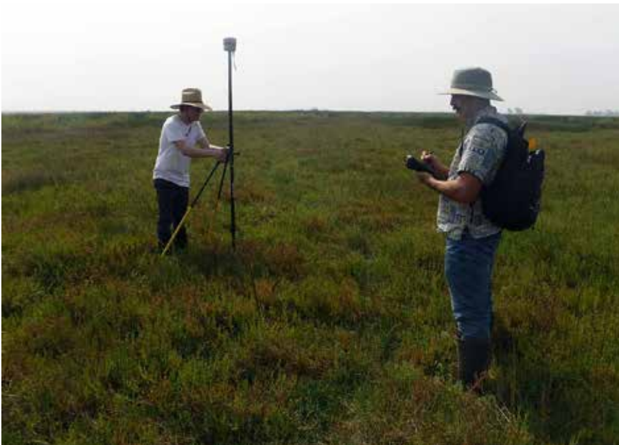
Dr. Kirk Waters and Jared Lewis, former Reserve Stewardship Coordinator, use the latest RTK instruments to conduct baseline vegetation sampling to inform a specially funded NOAA project to test UAV remote sensing technology for vegetation mapping at Rush Ranch. Photo: Michael Vasey.
