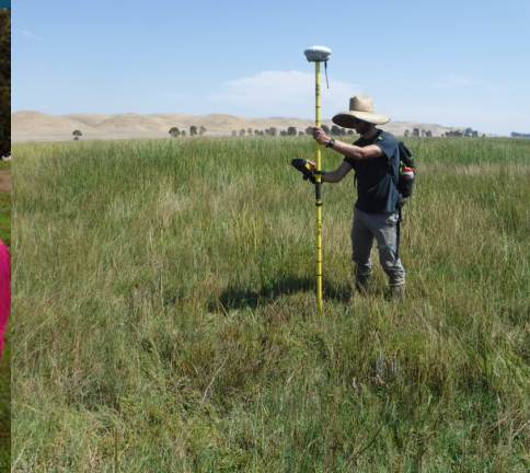
NERR tech using RTK GPS at Rush Ranch
