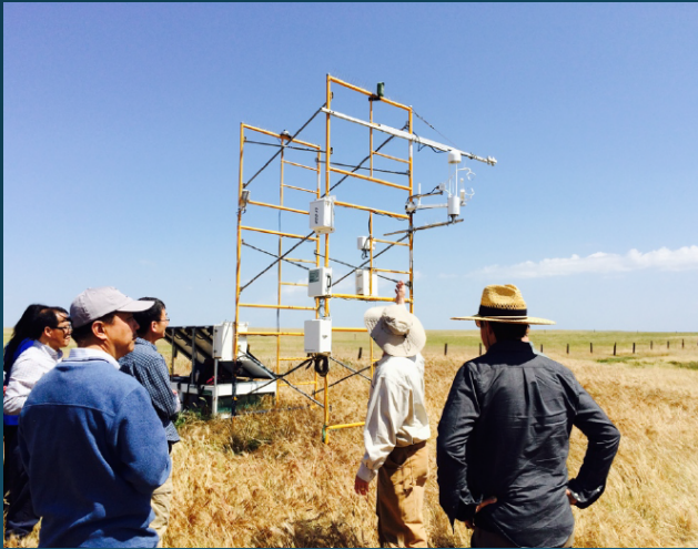
USGS eddy covariance flux tower measures methane emissions at Rush Ranch
