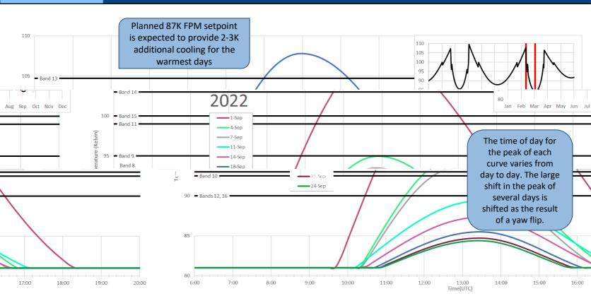
This plot shows hourly maximum temperature of the ABI focal plane module. The higher the temperature, the more saturated imagery becomes. Where the temperature rises to approach a black line for each band, marginal saturation may be observed in imagery. Where the temperature curve exceeds a black line for each band, the imagery may begin to saturate so much that it becomes unusable. The hour of peak temperature varies from day to day.
