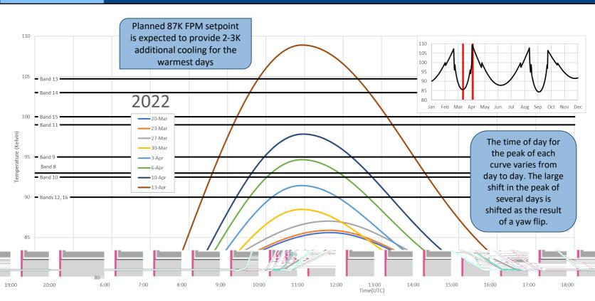
This plot shows hourly maximum temperature of the ABI focal plane module. The higher the temperature, the more saturated imagery becomes. Where the temperature rises to approach a black line for each band, marginal saturation may be observed in imagery. Where the temperature curve exceeds a black line for each band, the imagery may begin to saturate so much that it becomes unusable. The hour of peak temperature varies from day to day.
