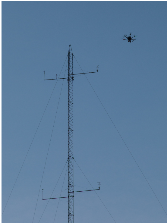
Figure 8. Drone parked next to the sonic anemometer at 70 m a.g.l.
