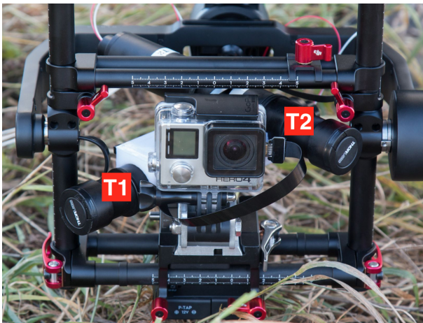
Figure 2. Gimbal payload: GoPro camera and two telescopes highlighted with T1 and T2 (here mounted with 90° opening angle between them) with protective lens caps. Picture taken from the photo gallery ( https://work.courtney.dk/#collection/364601 , last access: 28 January 2020).
