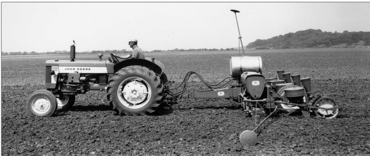
Figure 10. Tractor pulling implement, using cylinders permanently attached to the tractor.
