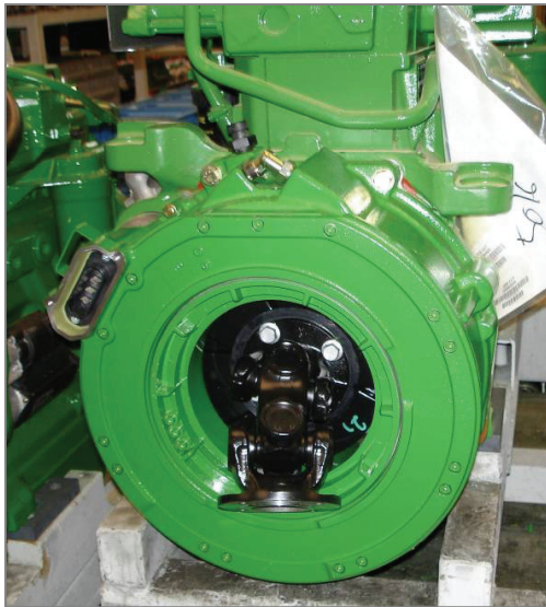
Figure 27. Flywheel mount AC induction generator.
