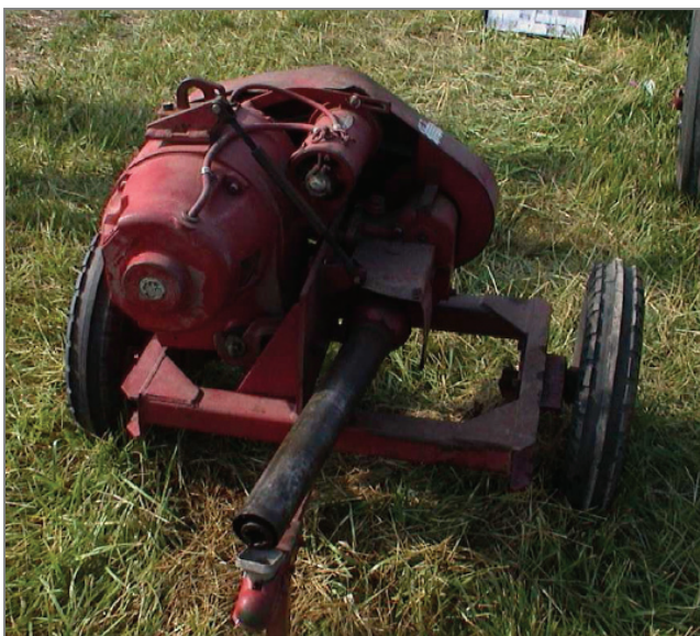
Figure 24. PTO-driven generator, retrofit power generation device.
