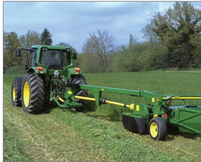
Figure 4. PTO driveline on mower conditioner, showing shields.
