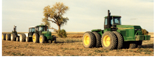
Figure 36. 4WD power hop test equipment in Colorado, 1991.
