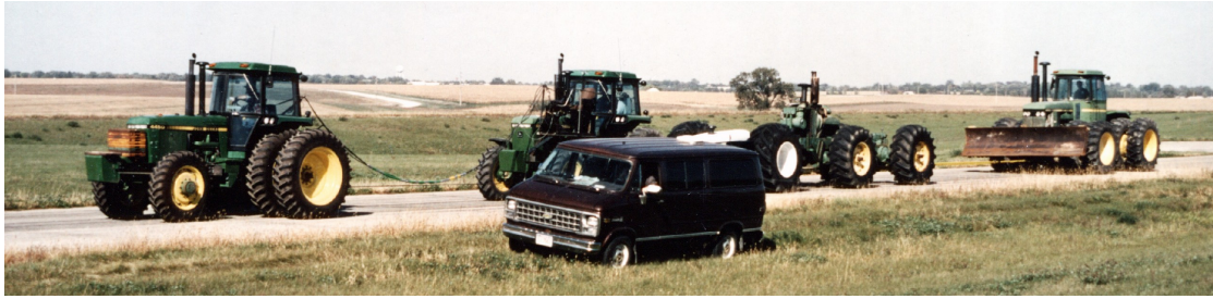
Figure 23. Test tractor, instrument tractor, and load units on concrete test track—1989.
