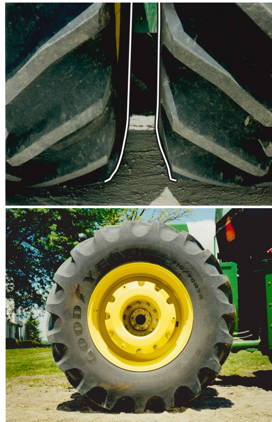
Figure 33. Overinflated radial tires.
