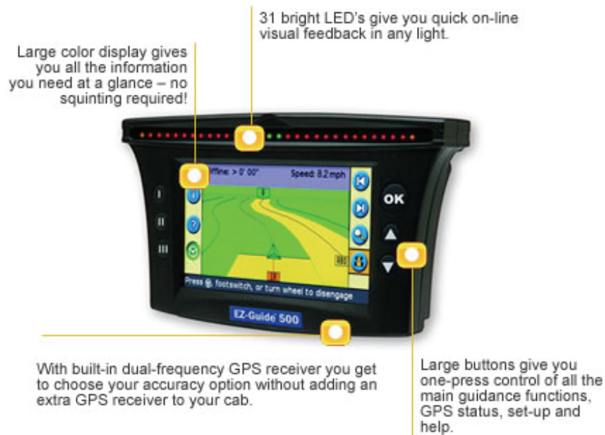
Figure 3.2. Modern full-featured manual guidance system: Trimble EZ Guide 500.
