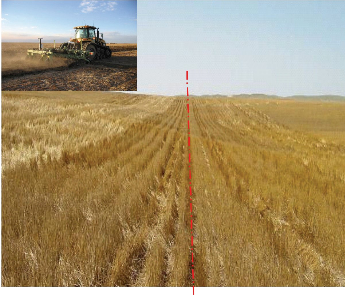
Figure 5.1. Test results of automatic vehicle and implement steering in a 12° slope field. Without automatic steering, the implement would have sagged down 60 cm. With implement steering, this is limited to 2.5 cm.
