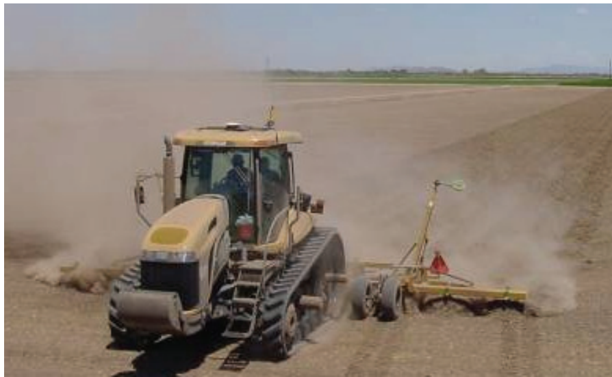
Figure 4.6. Caterpillar MT using automatic guidance over CAN network.
