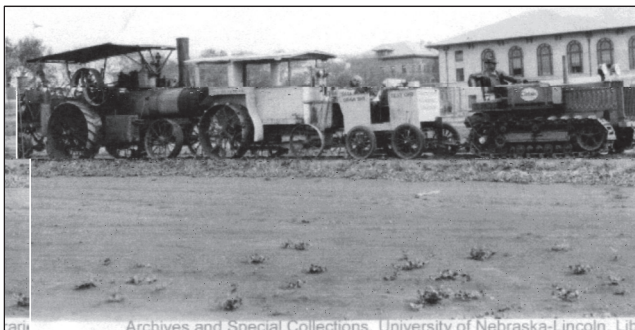
Figure 5. The second test car using a load tractor that is in turn pulling a steam tractor.
