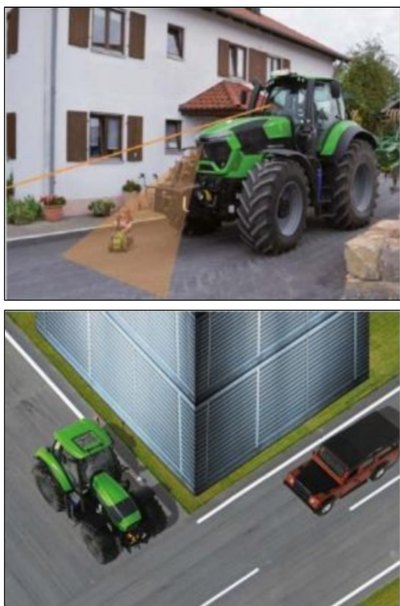
Figure 12. Driver Extended Eyes and panoramic view from cameras on a Deutz-Fahr tractor (source: https://issuu.com/ , Farming Precision Magazine).
