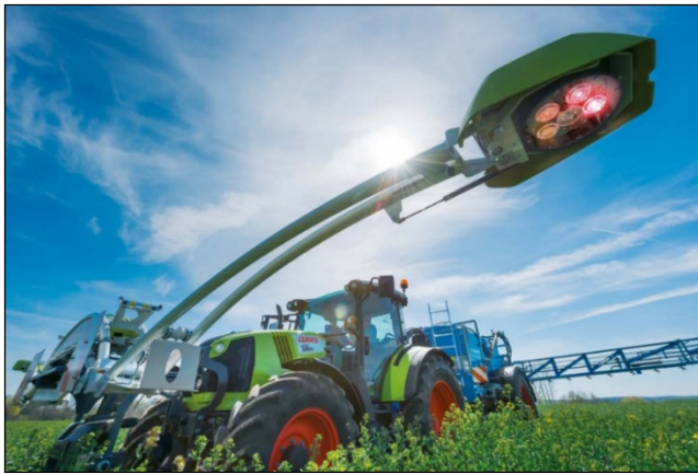
Figure 13. CLAAS ISARIA crop sensor (source: CLAAS, http://www.claas.com.au/products/easy/precision-farming/crop-sensor ).
