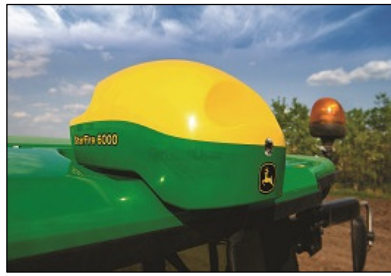
Figure 1. StarFire 6000 guidance system and terrain compensation (source: John Deere, www.deere.com.au).
