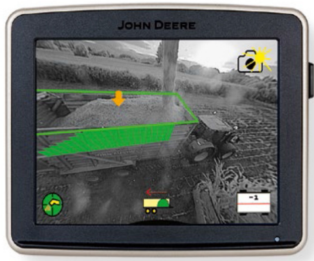
Figure 10. Machine vision (using a stereo camera system): Active Fill Control of transport trucks when forage harvesting (source: John Deere, https://www.deere.com.au/en/index.html ).
