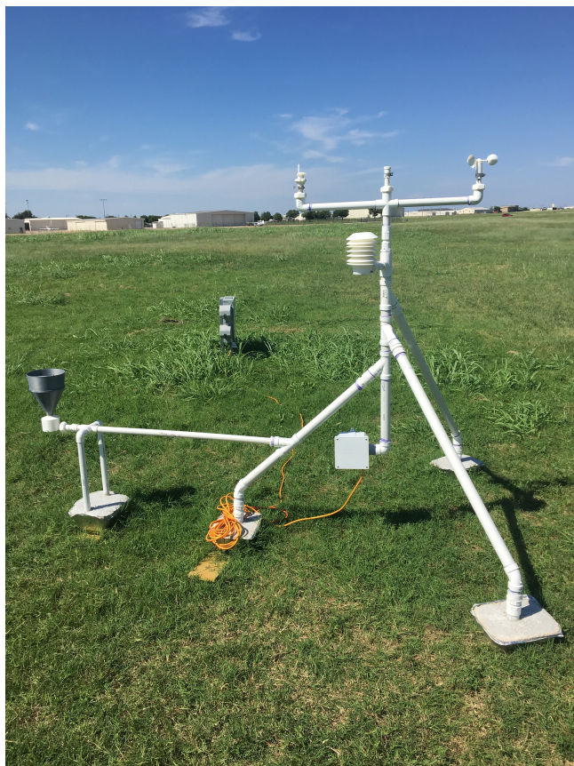
Figure 2. 3D-printed weather station upon initial installation in the field.
