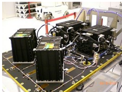
Figure 3 : OSTM/Jason-2 Posidon-3 Instrument
