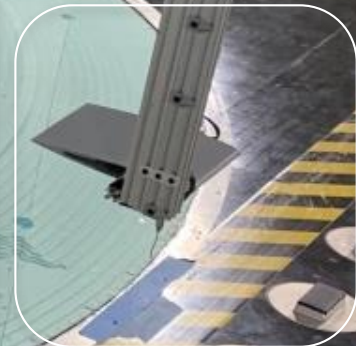
(b) Zoomed in view of the Cobra Probe over the topographic model surface
