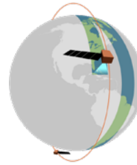
JPSS satellites travel in a polar orbit as the Earth rotates underneath.
