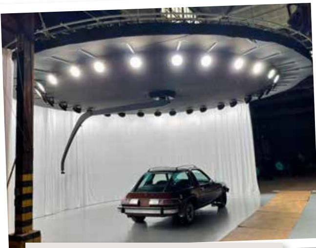
The Arc Eye Camera System was installed at the Collections Resource center to produce high-resolution 360 degree images of our large artifacts.
