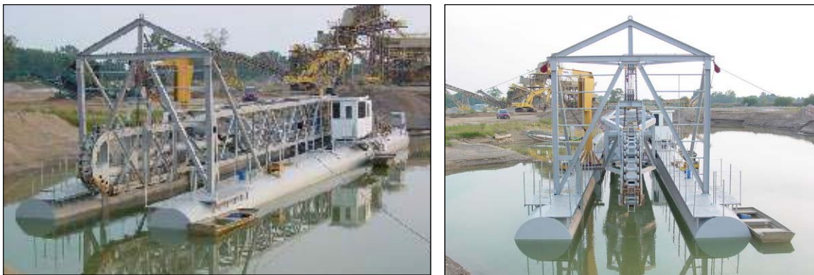
Figure 7. A 356 mm (14 in) sand and gravel dredge with linear cutter (Courtesy of Twinkle Company).
