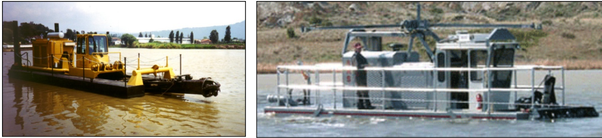
Figure 6. A 203 mm (8 in) discharge and 305 mm (10 in) suction fixed spud dredge (left) ( Courtesy of Dredgemasters International) and a Rotomite dredge (right) (Courtesy of Crisafulli).
