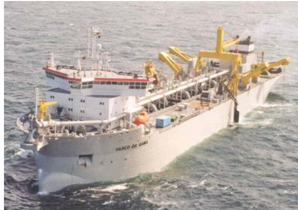
Figure 2. Trailing suction hopper dredge, Vasco da Gamma (Courtesy of Jan de Nul).
