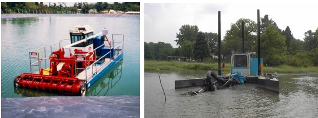
Figure 5. Small auger dredge (left) and a 203 mm (8 in) swinging ladder dredge with cutter head (right) (Courtesy of Ellicott and Dredging Supply Co., respectively).
