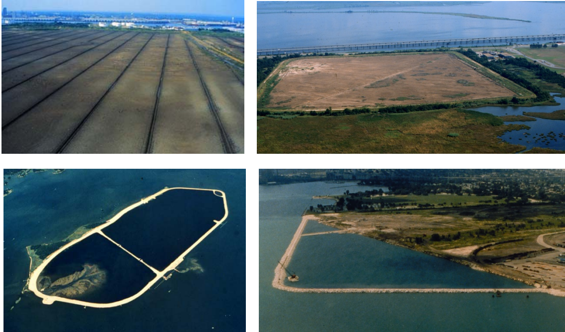
Figure 23. Example confined placement areas upland (top), island (bottom left), and near shore (bottom right). (Courtesy of Mike Palermo)
