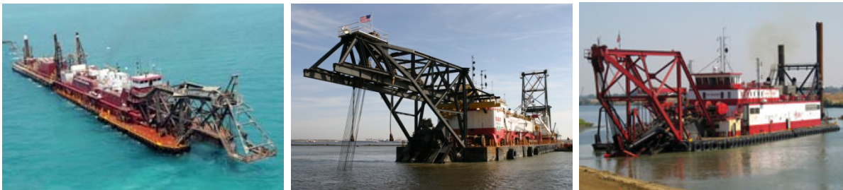
Figure 3. Large cutter suction dredges, Texas (left), RS Weeks (middle), and HR Morris (right) (Courtesy of Great Lakes dredge and Dock, Weeks Marine, and Manson Construction, respectively).
