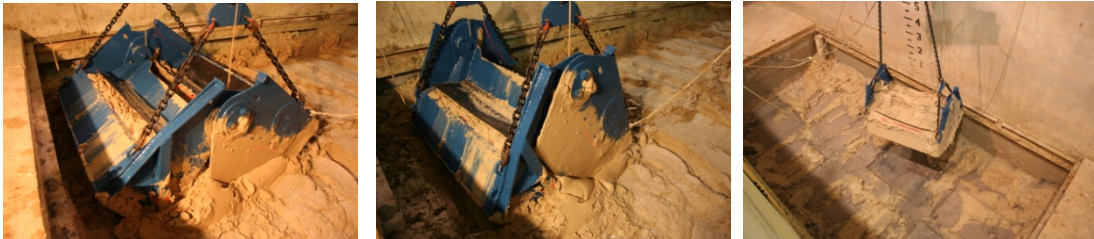
Figure 13. Laboratory environmental clamshell bucket constructed by CableArm Inc for the Haynes Laboratory at Texas A&M University.
