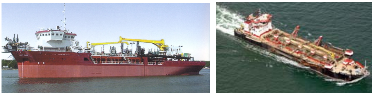
Figure 1. Trailing suction hopper dredges Liberty Island (left) (Courtesy of Great Lakes Dredge and Dock) and Glenn Edwards (right) (Courtesy of Manson Construction).
