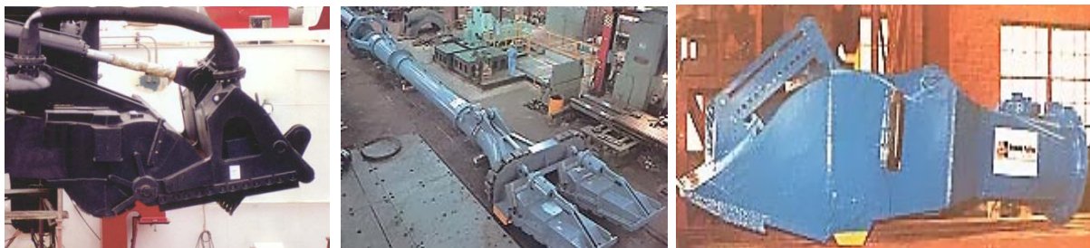
Figure 26. Common dragheads used by trailing suction hopper dredges.
