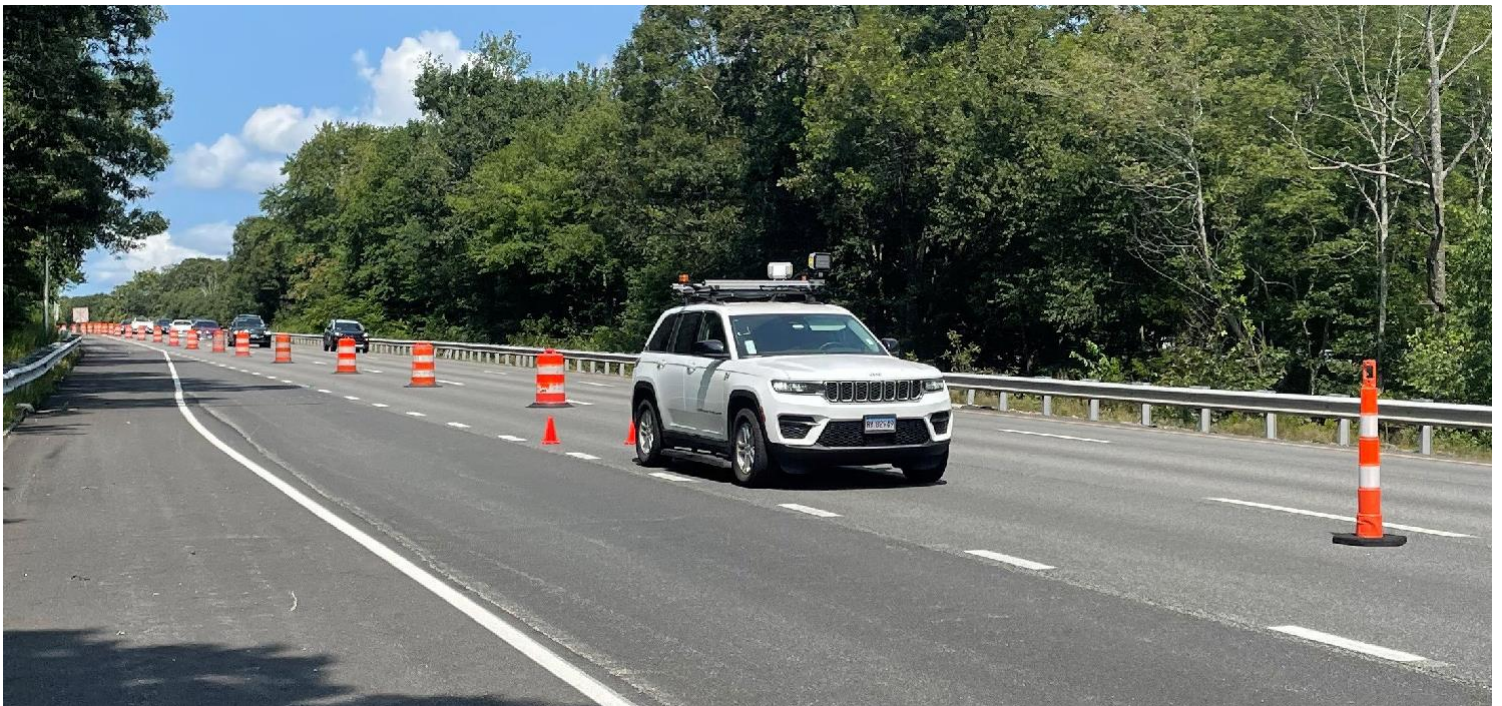
Figure 5 | Deployed technology monitoring vehicle speeds.
