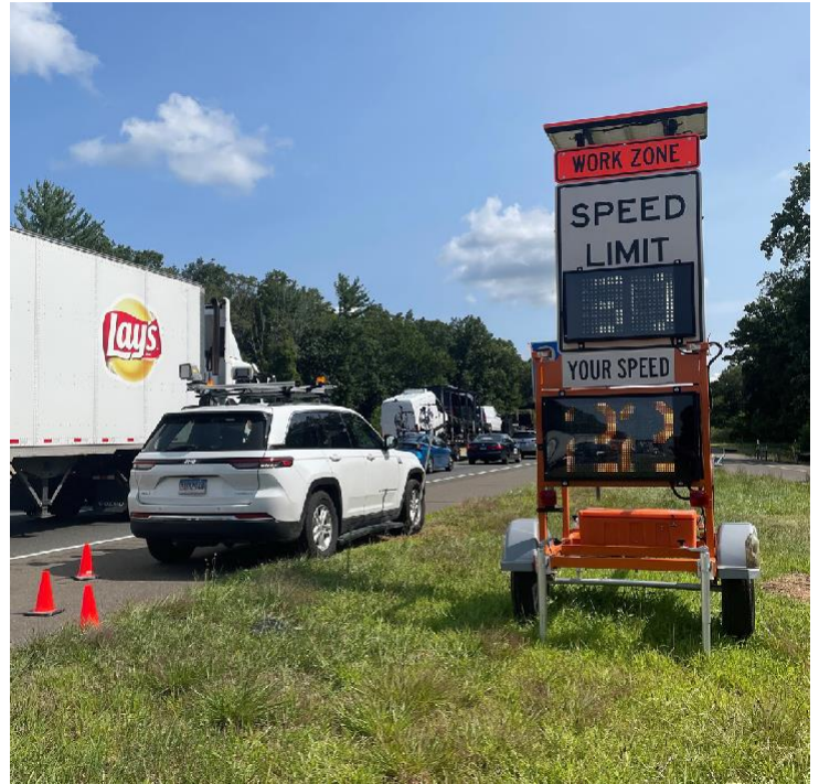
Figure 3 | Deployed technology monitoring vehicle speeds.
