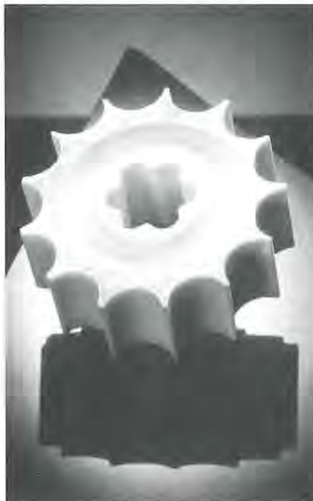
Desktop prototype. This part, produced by a method called laser sintering, illustrates a technique developed through NSF's Small Business Innovation Research Program. Introduced into the marketplace when the researchers' small firm was acquired by B.F. Goodrich, the technique will enable engineers, operating with off-site computers, to convert ideas quickly into hard-to-produce parts.
