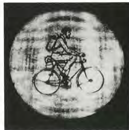
Novelty filter. Dana Anderson and Jack Feinberg collaborated on an ingenious new optical circuit that memorizes the shape and position of an object. A three-dimensional image of the object forms in the optical circuit—known as a “Novelty Filter”—but the image quickly fades unless the object moves or the background scenery changes, as seen in these two photos.
