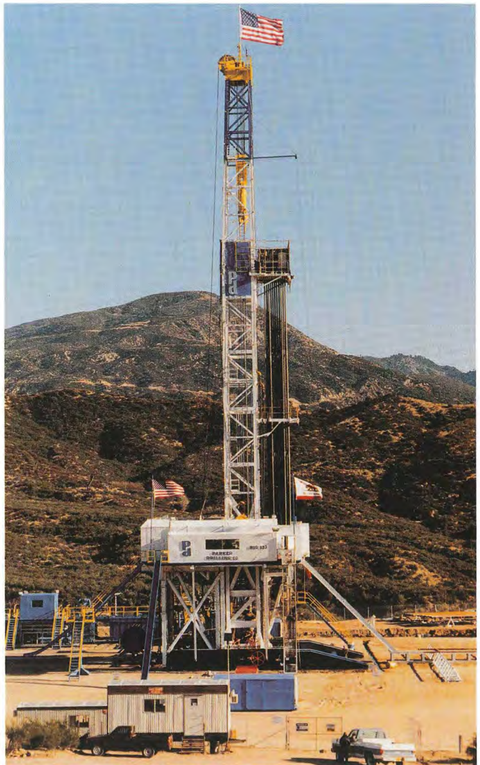
Earthquake research. At Cajon Pass, in the earthquake-prone region of the San Andreas fault in California, scientists have drilled a hole deep enough to sample the earth's crust and monitor the forces that may give early warnings of an earthquake.
