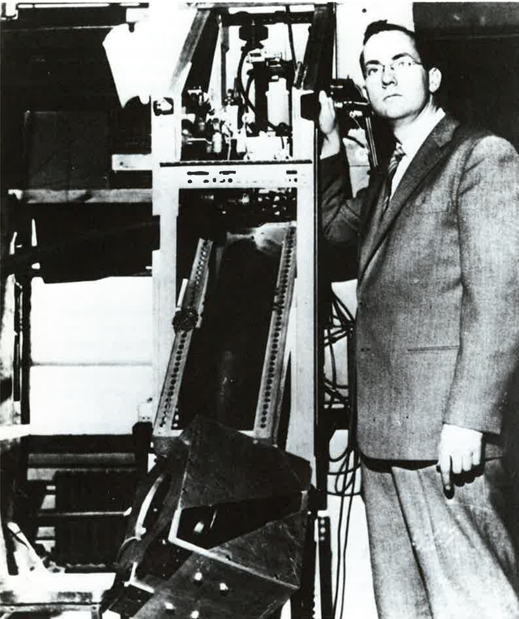
Early work. An early application of solid-state masers was in radio astronomy. Here Charles H. Townes stands beside the maser amplifier for the Naval Research Laboratory radio telescope. (Photo courtesy of AT&T Bell Laboratories)
