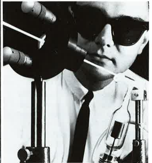
Laser progress. This is one of the first argon ion lasers. (Photo courtesy of Hughes Aircraft Company)
