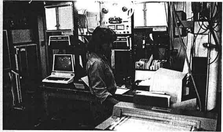
Studying warm-core rings. Research assistant from Woods Hole Oceanographic Institution monitors data displayed on a video screen aboard the R/V Knorr . She uses information from a huge multinet trawl (the MOCNESS), towed from the ship, to control the trawl's underwater operations. Drawing shows MOCNESS and other equipment used on the Knorr . These included pumps for work on plant pigments, two CTD/rosette sampler systems, 5-liter zooplankton grazing chambers, a 30-liter Niskin bottle, and a ring-net. (Note: XBT = expendable bathythermograph; CTD = conductivity/temperature/depth.)
