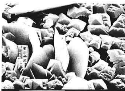
Photoconductors: Scanning electron micrograph shows a thin film of chlorogallium phthalocyanine. Phthalocyanines are substances that strongly absorb light in a region of the visible spectrum where the solar flux on earth is high. Working with thin films like this, chemists are making progress on ways to use such substances to convert light energy to electrical energy. (White line = 5 microns)
