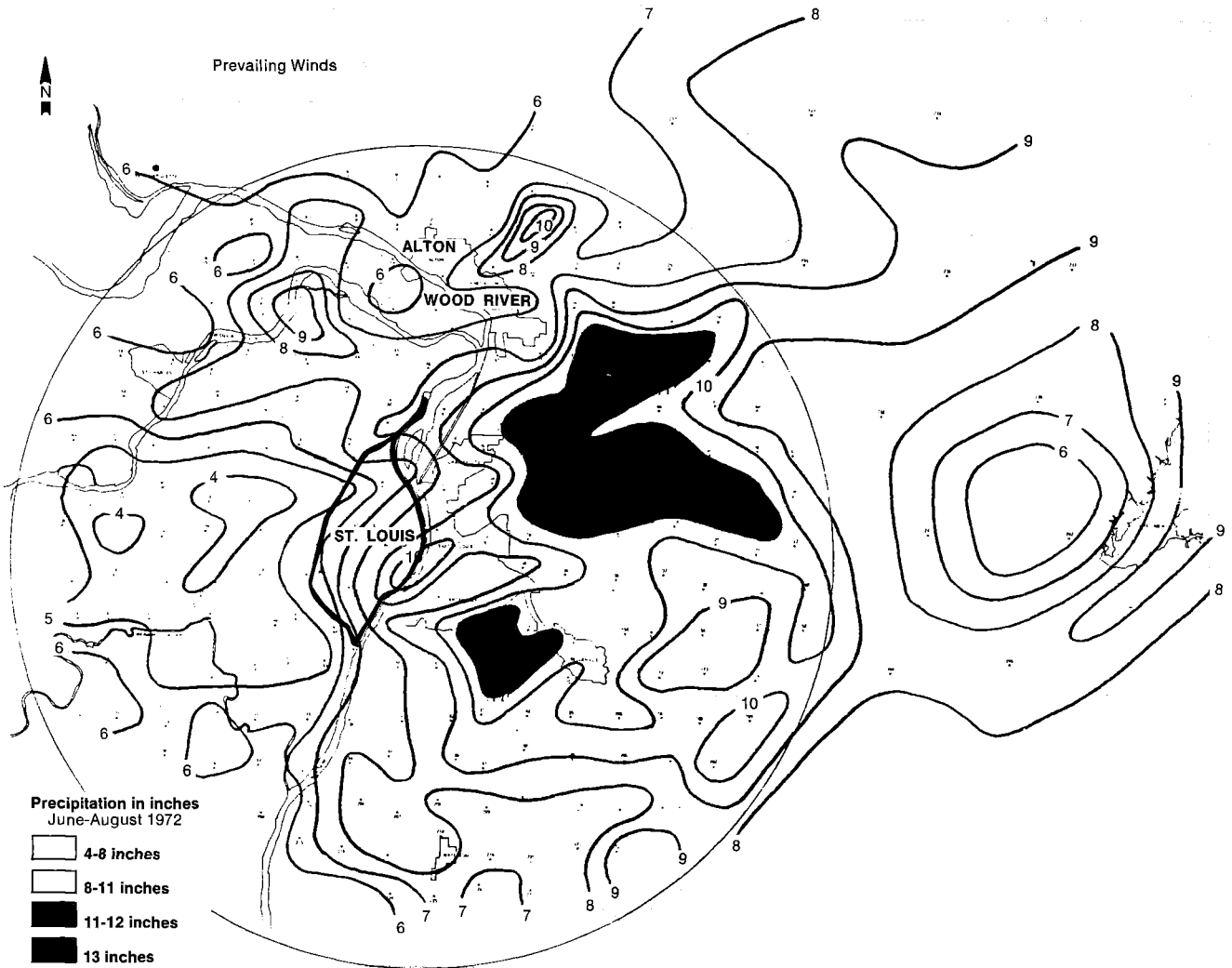
A precipitation map of the St. Louis area, based on measurements of rainfall taken during field operations June through August 1972, shows increased precipitation downwind of the metropolitan area.
