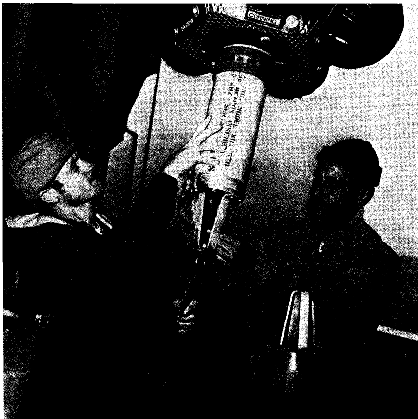
This sonar positioning beacon being inspected aboard D/V Glomar Challenger during Leg 19 in the Bering Sea is used as a reference on the ocean bottom in the system that keeps the vessel over a drilling and coring site. (Photo by Scripps Institution of Oceanography)
