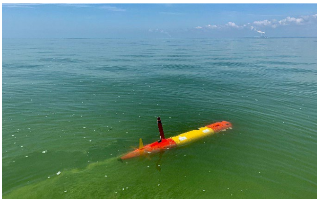
One of Monterey Bay Aquarium Research Institute's long-range autonomous underwater vehicles makes its way through the green, algae-rich waters of Lake Erie to track the 2019 harmful algal bloom as part of a research collaboration with NOAA. (Credit: Ben Yair Raanan, Monterey Bay)
