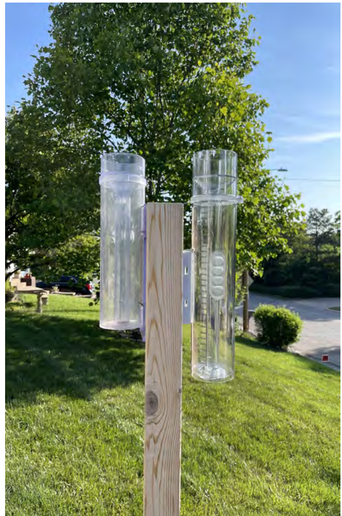
Stratus (L) and TROPO (R) rain gauges. KS-RL-64.
