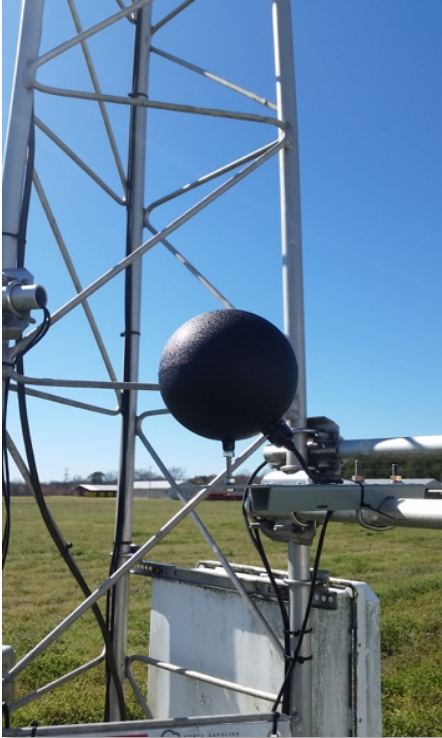
Black Globe Thermometer used to calculate heat stress in Rocky Mount
