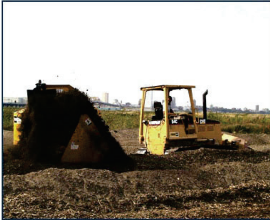
Figure D-15. Scat turner maintaining compost piles.
