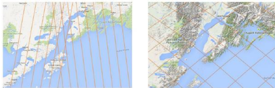
Figure 4. The orbits along the tracks of Cryosat-2 over a three day period (left) and Jason-2 over a ten day period (right).
