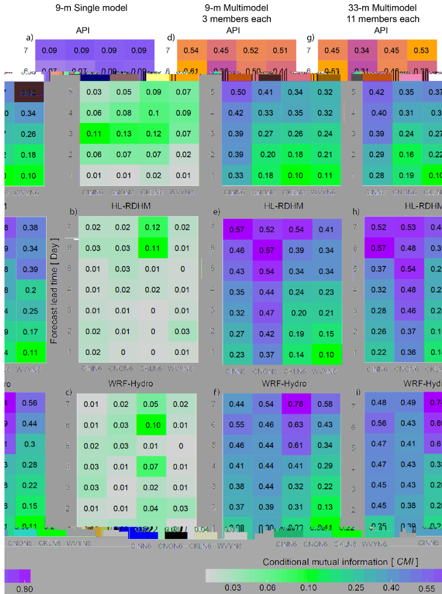
Figure 6. CFI of the ensemble streamflow forecasts versus both the basin and forecast lead time for three different experiments: a-c) 9-m single model, d-f) 9-m multimodel, and g-i) 33-m multimodel forecasts. The 9-m single model experiment consists of a 3-member single model forecast from one of the hydrological models combined with a 6-member ensemble from the same model. In the 9-m multimodel experiment, a 3-member single model ensemble forecast from one of the models is combined with a 6-member ensemble from the remaining other two models (3 members from each model). The last experiment, 33-m multimodel, is the same as the 9-m multimodel experiment but using instead 33 members (11 members from each model).
