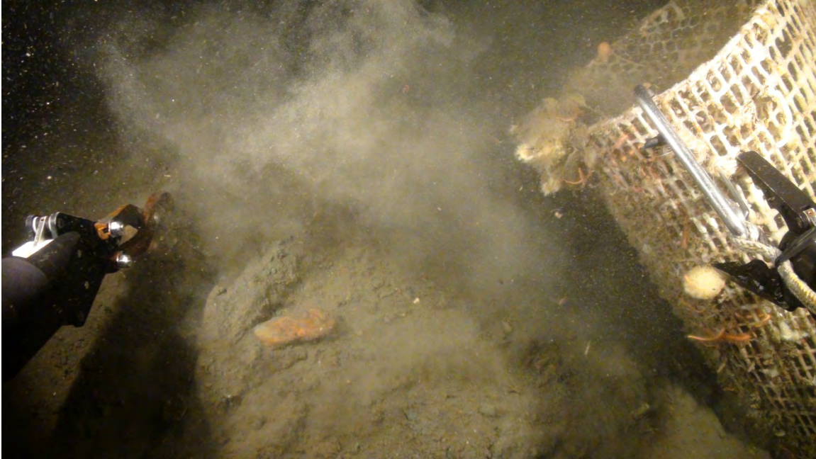
Figure 20. HD image of the ROV hooking the cylindrical trap with the carabineer.
