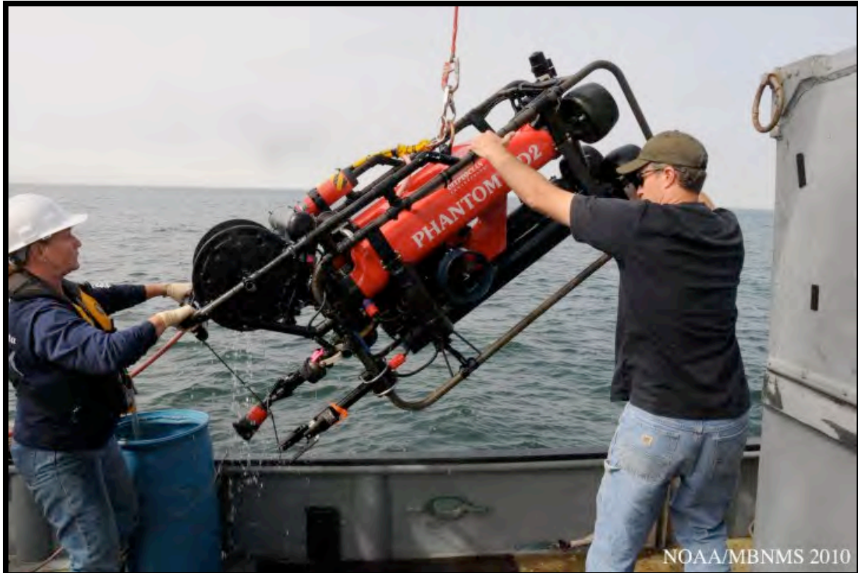
Deck Manager Donna Kline and ROV Pilot Andy Lauermann land the Phantom HD2 ROV safely back onboard the Fishing Vessel Donna Kathleen. The ROV is used to locate the fishing gear targets, and then using a hook attached to a manipulating arm, it clips onto the gear. The spool line (located above the arms) will feed out line as the ROV is retrieved, and then the line is transferred over to the boat winch and the gear is hauled up on to deck.
