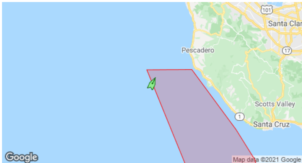
Figure 5. Example map included in a Marine Traffic notification. The green icon is the vessel and the red box is the customized alert zone.
