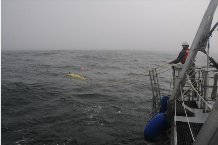
Figure 21. Deployment of the AUV. The AUV is not released until after confirming that we have communication with it to share navigation data.
