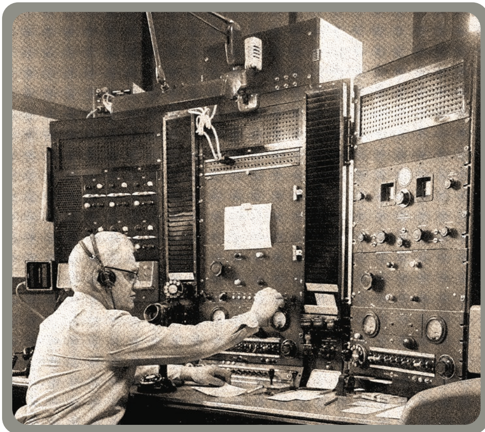
Albert Klopp, manager of Lorain Electronics Corporation's Station WAS in Duluth, adjusts the controls of his 1,000-watt transmitter in 1972. Klopp led a team of three operators who connected radio-telephone calls to ships sailing the Great Lakes.
